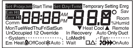
Fig. 5. Display of all the segments of the LCD.
