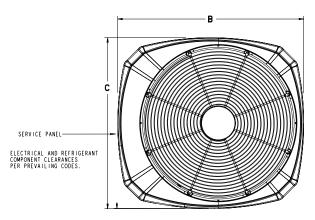
TOP DISCHARGE AREA SHOULD BE UNRESTRICTED FOR AT LEAST 1524 (5 FEET) ABOVE UNIT. UNIT SHOULD BE PLACED SO ROOF ROUN-OFF WATER DOES NOT POUR DIRECTLY ON UNIT, AND SHOULD BE AT LEAST 305 (12") FROW WALL AND ALL SURROUNDING SHRUBBERY ON TWO SIDES. OTHER TWO SIDES UNRESTRICTED.
